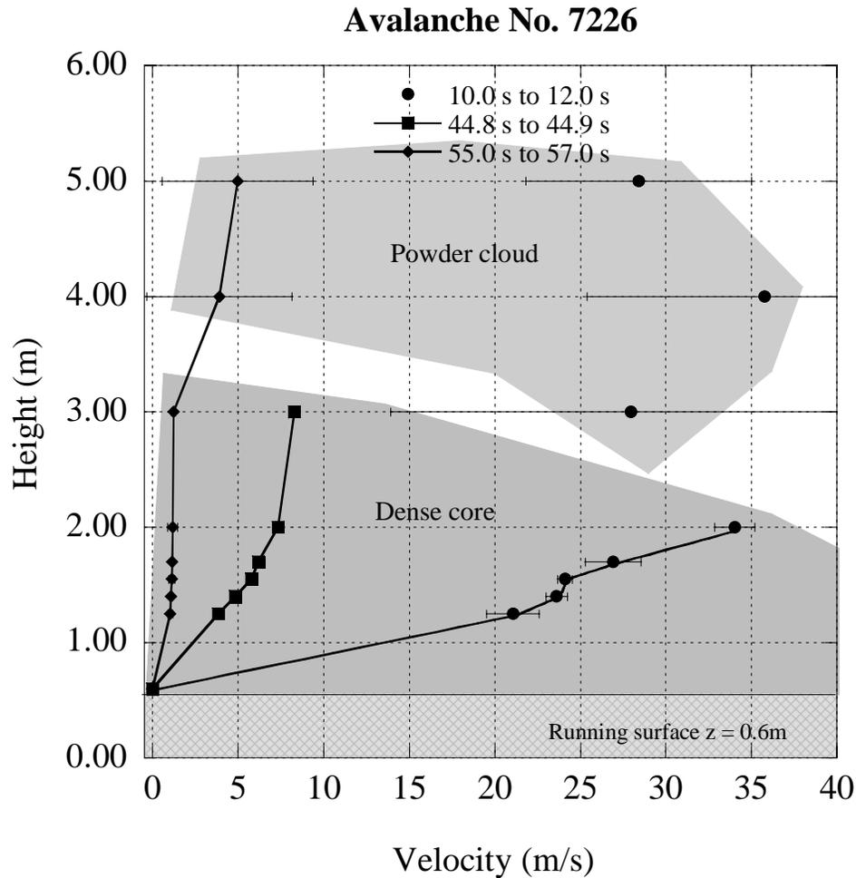
Figure 2: Distribution of avalanche velocity with height for three different time periods for a medium sized mixed flowing/powder avalanche from the Swiss Vallée de la Sionne test site.
