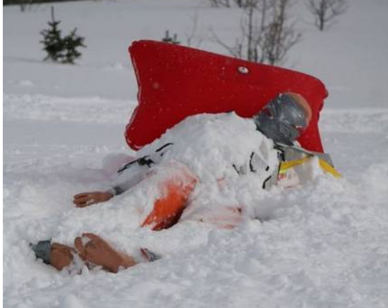
Figure 2: JTW Associates Dummy airbag testing in British Columbia during winter 2007/2008. Photo courtesy of JTW Associates.
