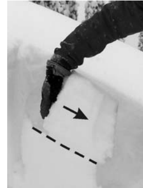
Figure 4: Hand shear test. A column, approximately 30 cm by 30 cm, is isolated about 40 cm deep by hand or with a ski pole. The column is manually pushed downslope and any slope parallel fractures noted.
