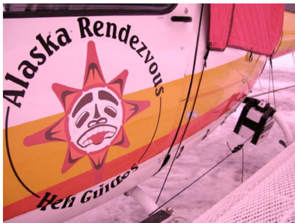
Figure 4: Helicopter mounted FMCW radar measurements. 12-18 GHz radar is white box bolted to arm of skid.
