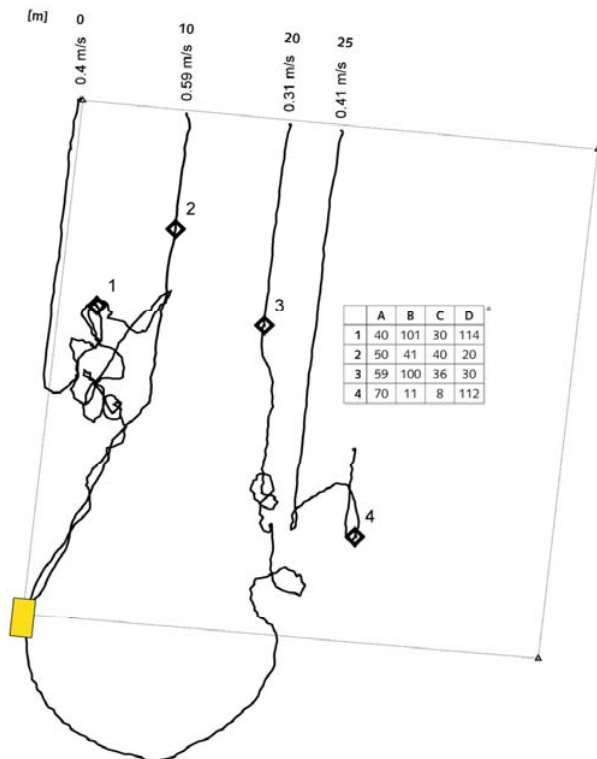
Figure 4: Trajectories of a beacon with no useful range with a horizontal transmitter in a good coupling position
