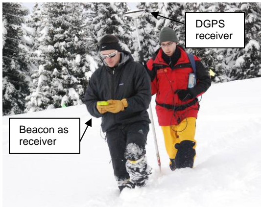
Figure 1: The searcher was directly followed by a second person with a DGPS receiver.
