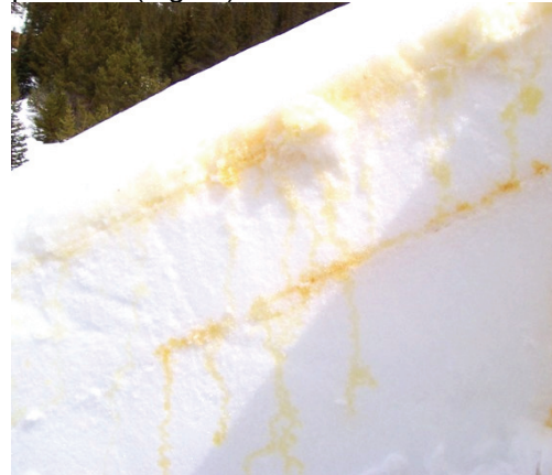
Fig. 13: Vertical and planar wetting in moist fine grained snow.
