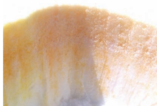
Fig.14: More uniform wetting in older, large, coarse grained, mature, output snowpack
